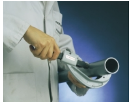
Cutting the pipe to length
